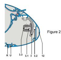
changed, the front profile (Fig. 2 no. 12) must be reset if necessary to ensure that the cassette closes properly.
